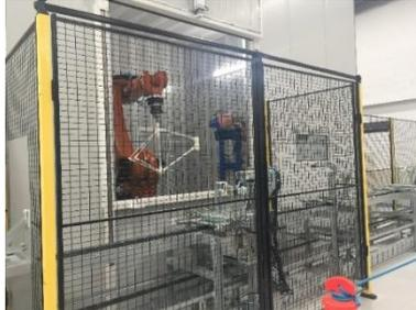
Moreover, Titomic Kinetic Fusion process could create some complex shapes, such as oval, tear-drop and conical tubes with no limited build size while limited build size and product shape could be produced by traditional additive manufacturing process. Apart from that, the whole process neither requires inert environment nor metal melting, which could eliminate oxidation issues and save up to 80% of material wastage.
