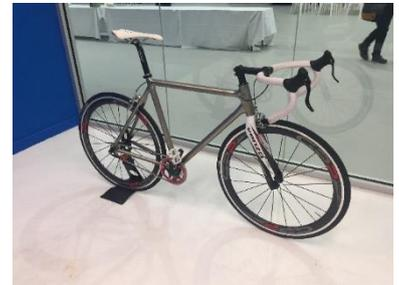
The build time for one Titanium bicycle frame will be 30 minutes by Titomic, which is much shorter than five days using traditional additive manufacturing.
